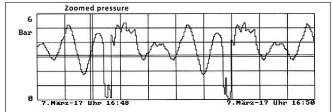
Synthetic material; DN 40 house pipe; LD Pulse in the house; sensor on the LD-Pulse
