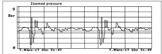
Cast iron; DN 125 main pipe; LD Pulse on hydrant; sensor on the LD-Pulse
