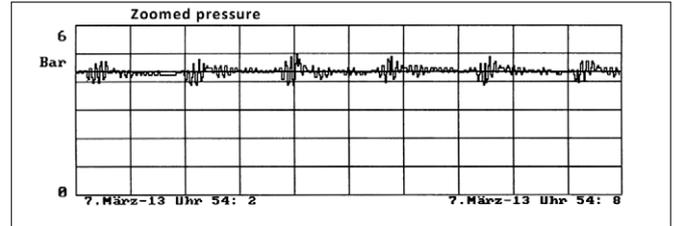
Synthetic material; DN 100 main pipe; LD Pulse on hydrant; sensor in 55 m
