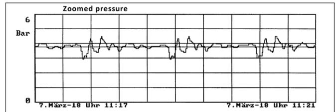
Cast iron; DN 125 main pipe; LD Pulse on hydrant; sensor in 55 m
